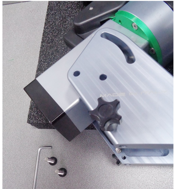
Remove the latitude adjustment bar and place it in the required position on depending on the user latitude observatory location.
